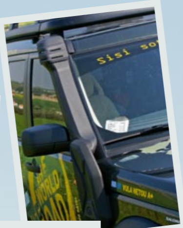
Snorkel, protective sliders and 10mm sump shield.
