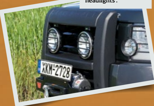
Bullbar with auxiliary headlights.
